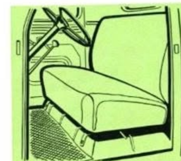
The manually controlled lever allows a three-inch seat adjustment, a feature much appreciated by drivers. In this view the seat is in rear position.
