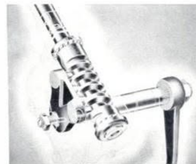
A vital factor in easy handling and safety at all speeds is the improved cam-and-twin-lever type steering mechanism. Both the steering cam and the twin levers are fully enclosed in an oil and dustproof housing and constantly operate in lubricant.
