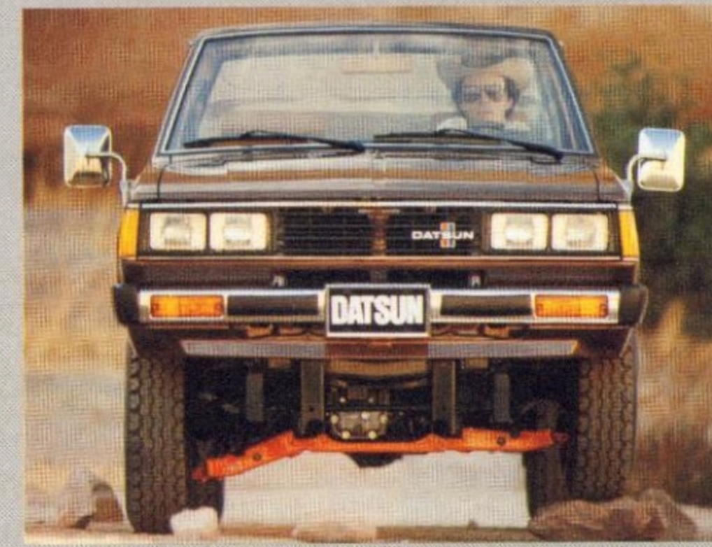
Independent front suspension, showing maximum travel.
