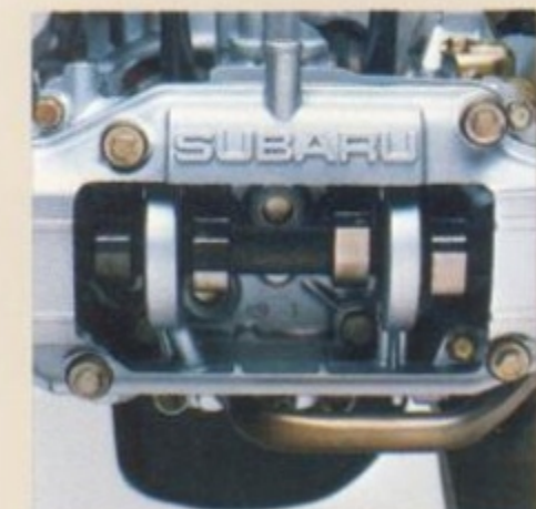
Turbocharged overhead cam engine (cut-away view) provides a reserve of extra performance.
