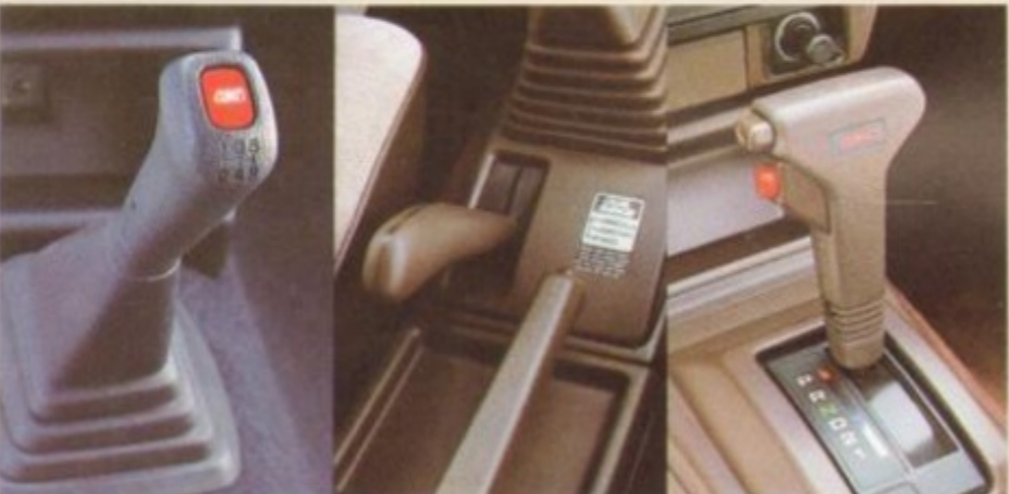
"On Demand" 4WD 5-speed transmission. "On Demand" 4WD Dual Range 5-speed transmission. "On Demand" 4WD automatic transmission.
