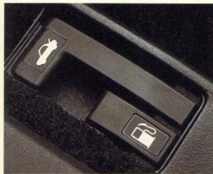
Remote releases allow the driver to open the hatch or fuel filler door of the Civic Hatchback without ever leaving the car.
