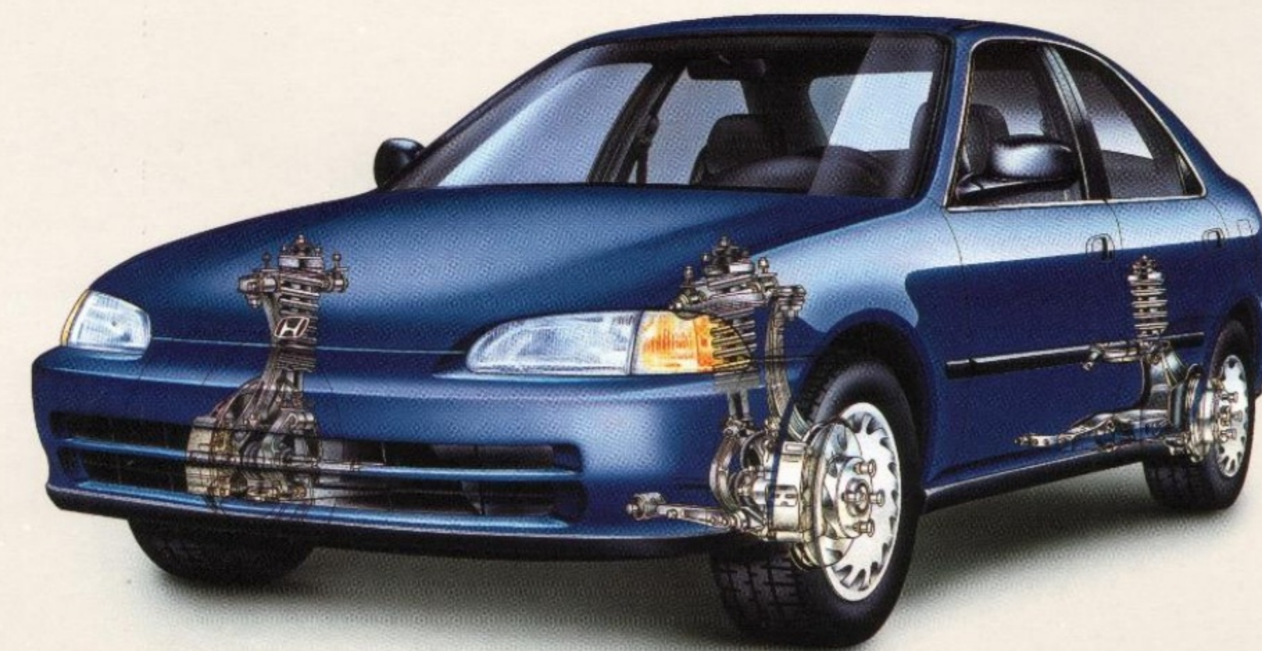
Civic's 4-wheel double wishbone suspension and longer wheelbase soak up bumps and road disturbances.
