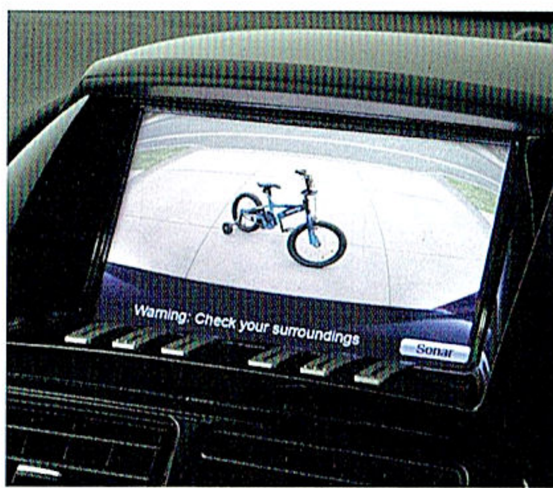
Reverse camera.* Activates automatically when the car is engaged in reverse gear. With a fisheye lens capable of providing a 130° wide angle view up to 10 metres behind the car.
