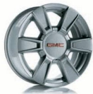
A – 17" x 7" painted aluminum, standard on all models
